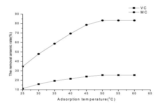
Fig.7: Effect of the adsorption temperature. Experimental condition: 30mL 0.3g/mL of soil alkali, t=40minand 0.07g pH7 MC or pH7 VC. Other experimental conditions were described procedures.
