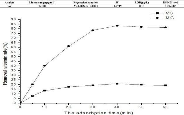
Fig. 5: Effect of the adsorption time. Experimental condition:30mL 0.3g/mL of soil alkali ,0.07g pH7 MC or pH7 VC,T=50 °C.Other experimental conditions were described procedures.
