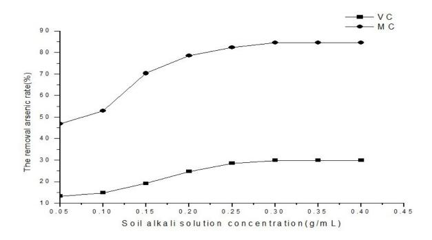
Fig.4: Effect of soil alkali solution concentration. Experimental condition: 0.07g pH7 MC or pH7 VC, t=40min and T=50°C. Other experimental conditions were described procedures.
