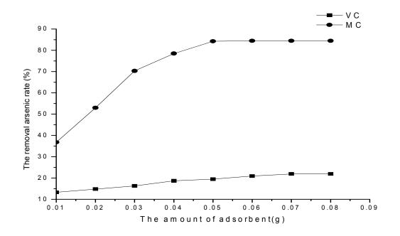
Fig.8: Effect of the amount of adsorbent. Experimental condition:0.07g pH7 MC or pH7 VC,30mL 0.3g/mL of soil alkali, t=40min and T=50 °C.Other experimental conditions were described procedures.
