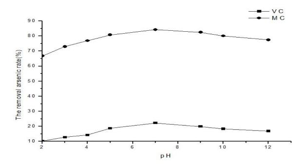
Fig.6: Effect of pH. Experimental condition: 30mL 0.3g/mL of soil alkali, t=40min and T=50°C. Other experimental conditions were described procedures.
